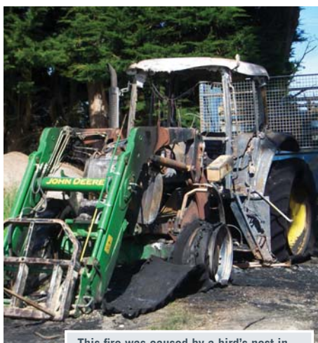
This fire was caused by a bird's nest in the engine built during the course of a lunchtime. (The tractor was checked that morning). The driver was unharmed.
