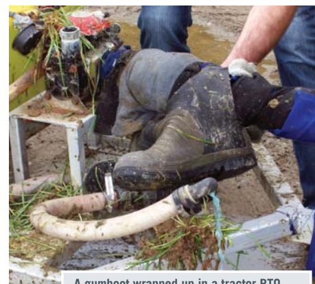
A gumbboot wrapped up in a tractor PTO shaft is a graphic demonstration of how quickly farm accidents can occur. The farm staff member suffered serious leg injuries, but was fortunate to escape alive.
